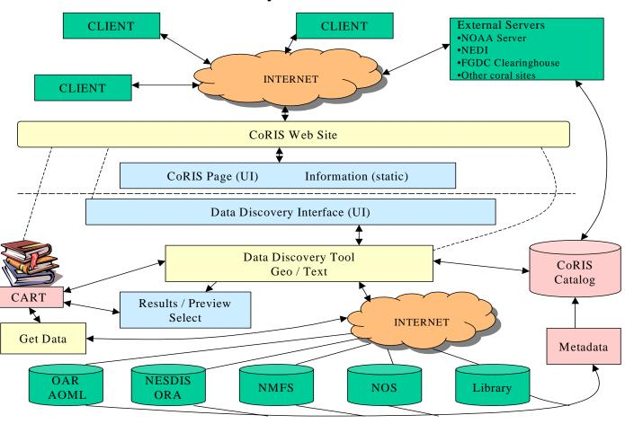
Figure 1 - CoRIS system architecture design
