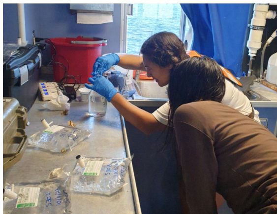
Figure 3: Scientists transfer discrete water samples collected from Subsurface Automated Samplers to Borosilicate glass bottles to transfer back to the lab for carbonate chemistry analysis.
